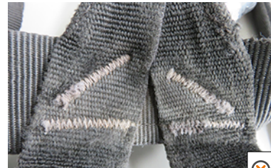
• Damaged safety stitching
